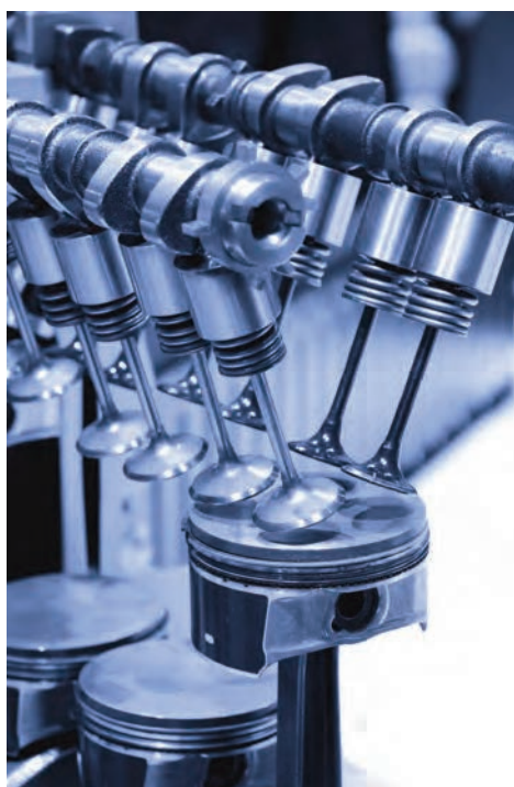
The interface between cylinder bore and piston contribute 45% of an engine's total frictional losses.
