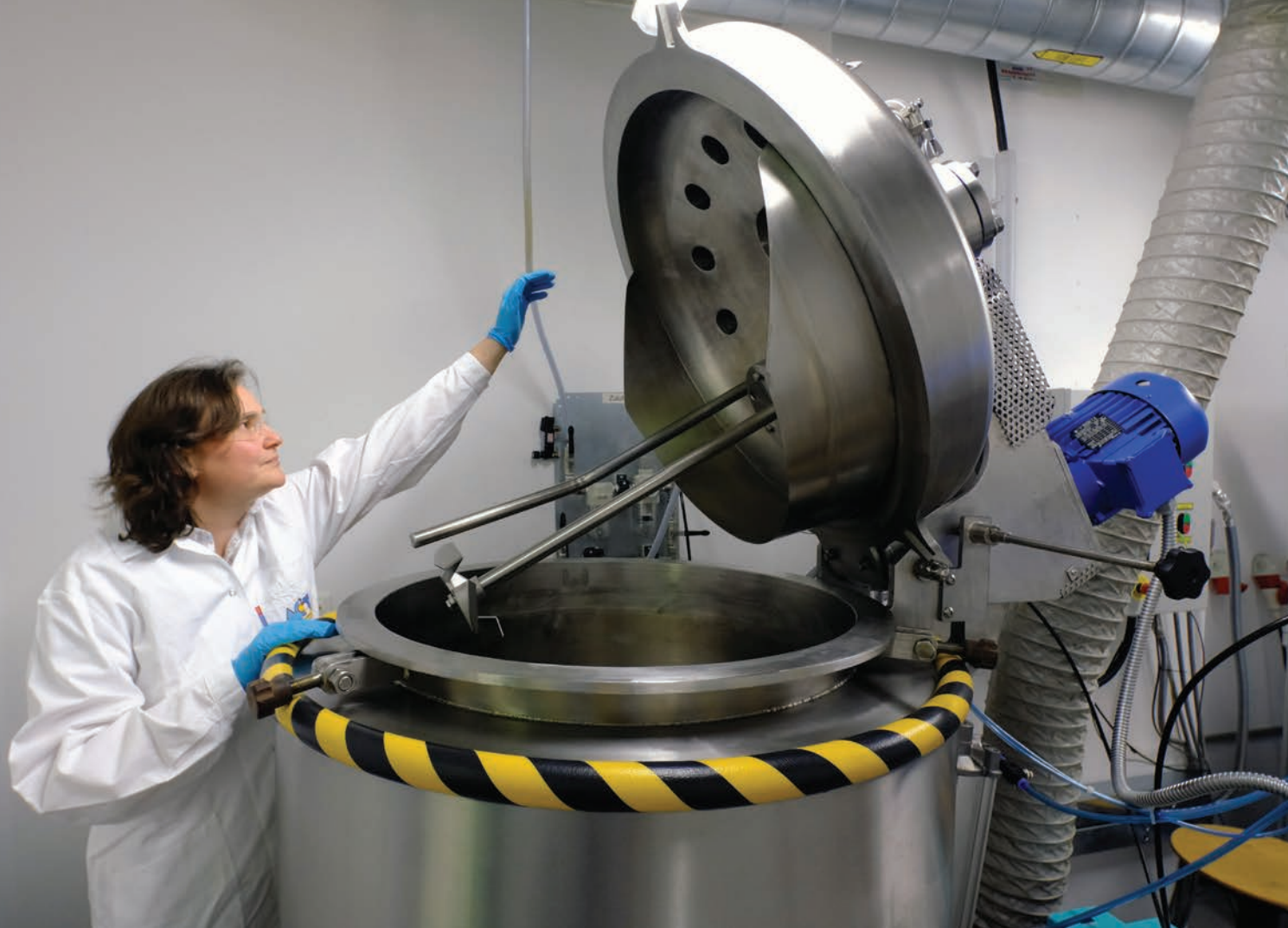
Large-scale device for lubricant aging to produce test oils with defined used oil properties, up to 200 L per batch possible. Photo courtesy of AC 2 T.
